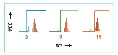
Using selective condensation growth methods in the Scanning Condensation Particle Counter, the STPC3 provides three cumulative size channels. In very clean liquids, the 15 nm channel measures native particles and the 3 nm channel is dominated by precursors, while the 9 nm channel is intermediate of these limits.
