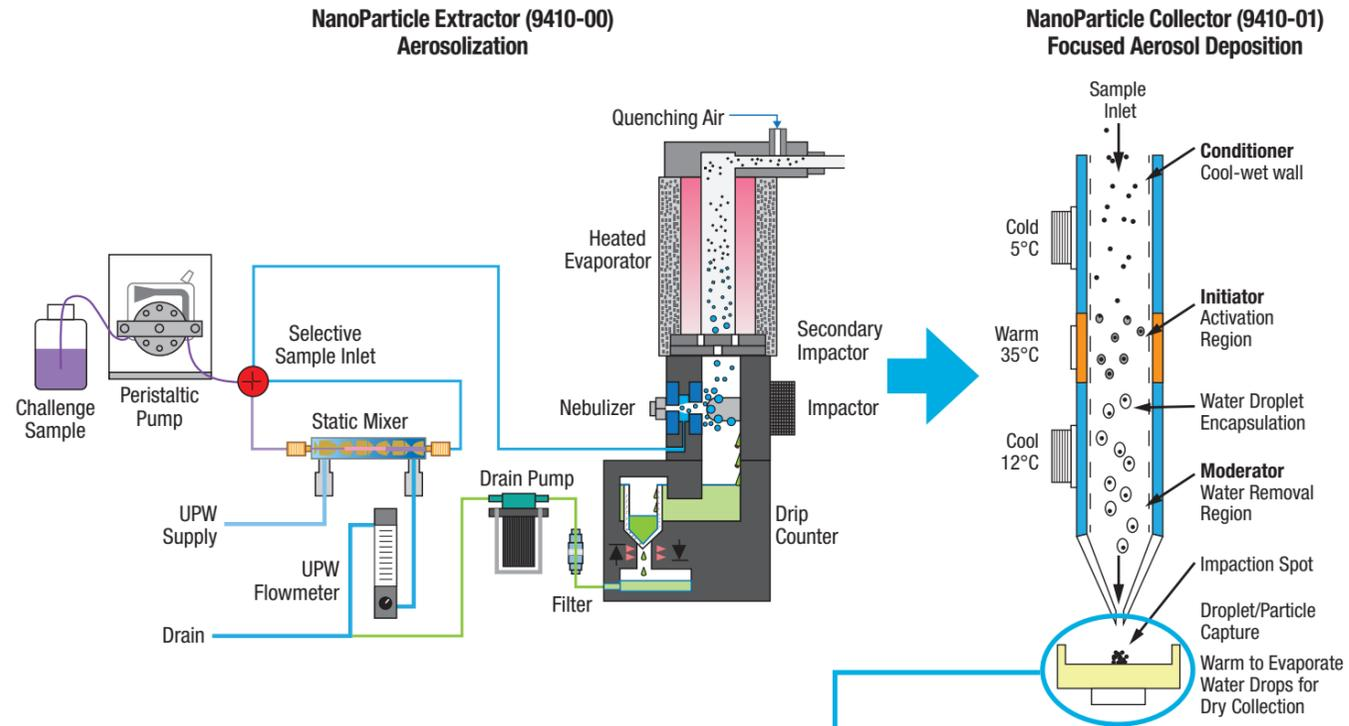
While the semiconductor industry has been able to count nanometer sized particles for decades it has struggled to identify the elemental composition of the particles. When a “particle event” affecting semiconductor yield occurs in a semiconductor manufacturing facility, knowing the composition of the contaminating particles can be crucial in identifying the source of the event and eliminating the problem.
