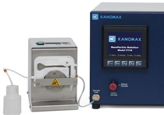
13. On the front panel of the NPE, turn the **Sample Selector** valve to **Diluted Sample**.
