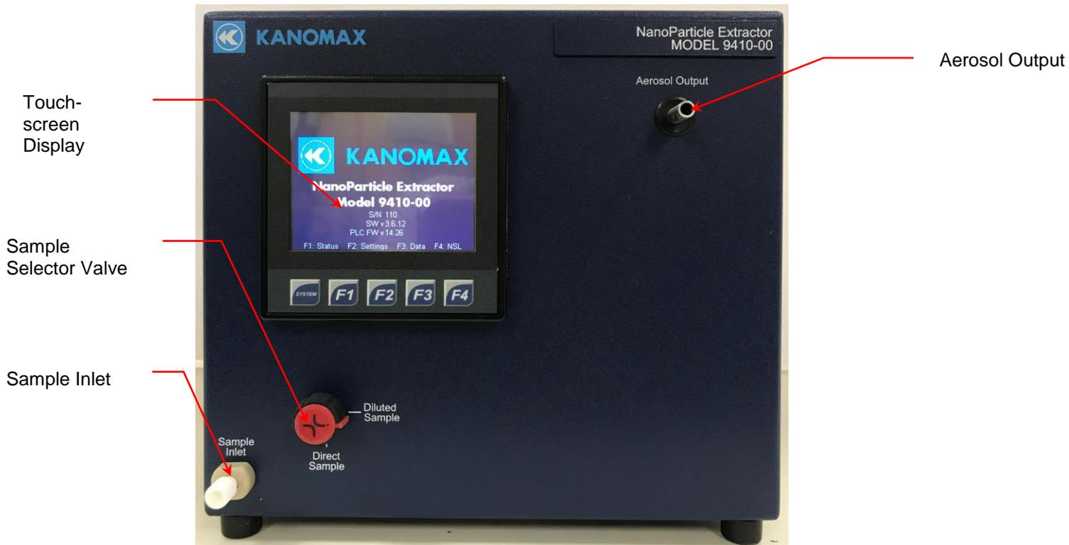
The Nano SpotLight is operated using the touch-screen display and the F1, F2, F3, and F4 buttons. The F buttons perform the following functions:
