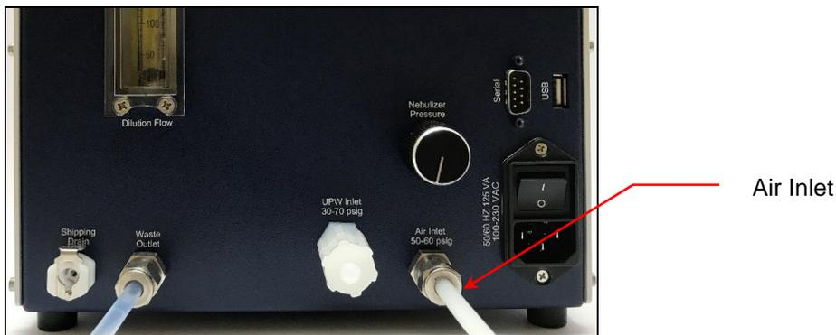
3. Using an adjustable wrench, tighten the Swagelok nut one turn past hand tight to swage the ferrules onto the tubing. Once the ferrules have been swaged, the fitting only requires slight tightening upon reassembly.
