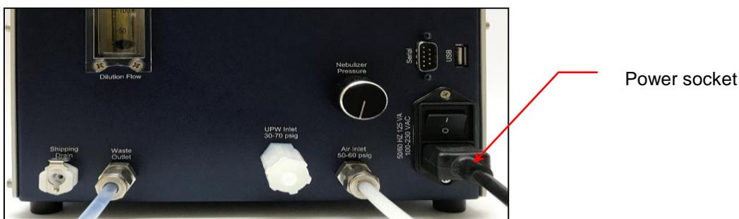
2. Plug the cord into an earth-grounded AC power source (100 to 240 VAC, 50 to 60 Hz, 0.6 A).
