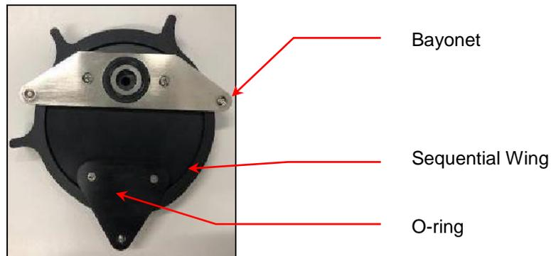
**Figure 20: SEM Sequential Sampler Bayonet Assembly.**
