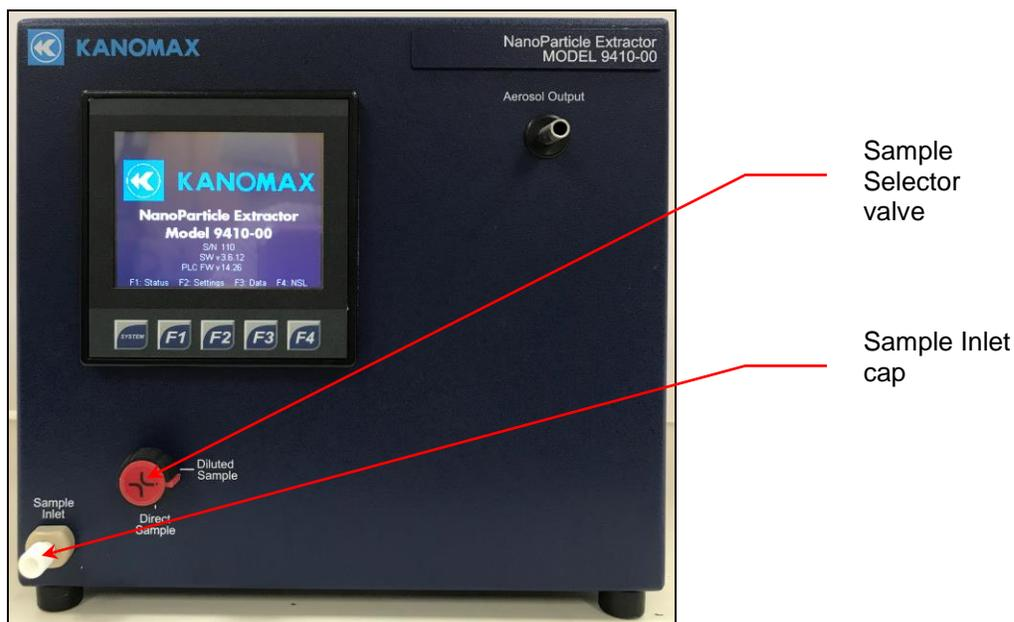
2. Remove the 1/4-28 plug protective cap from the **Sample Inlet** fitting.
