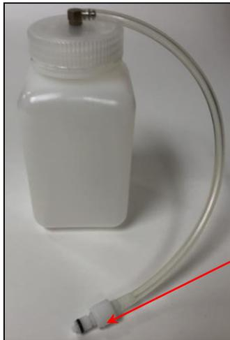
2. Push the connector into the WASTE WATER fitting.
