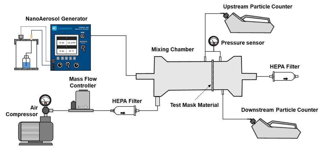
To the left is a schematic of the facial covering efficacy evaluation system. The NAG generates monodisperse PSL particles of 100 or 300 nm at an aerosol flow rate of 1.7 LPM, which mixes with a dilution flow of clean dry air into a 13.15 or 85 LPM total test flow in a 2.87-inch ID aluminum mixing chamber with 12-inch in length.
